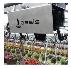
The OASIS module attaches to any existing or new hanging basket conveyer, such as ECHO or Boomerang, converting it to a weight-based watering system. The grower establishes the ideal weight of a watered basket, programs it into the system and the computer does the rest. It also stores your irrigation data for future analysis. You can control plant growth without PGRs, water heavier when you're about to ship and manage your basket watering from a phone or tablet. www.controldekk.com
