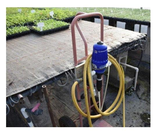
A calibration check is the easiest way to make sure your injector is hitting its mark. To do this, you'll need the injector (of course), an EC meter, your favorite fertilizer and a cup or beaker for sample collection.
